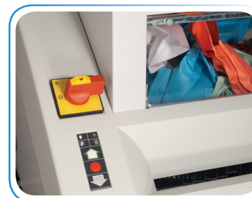
Easy-to-use control panel and lockable on-off switch
