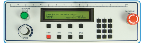
Control panel with LCD Display and 4 programmable jobs
