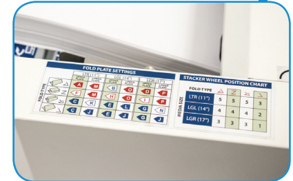
Fold guide icons match those on the fold plates, for intuitive, easy setup
